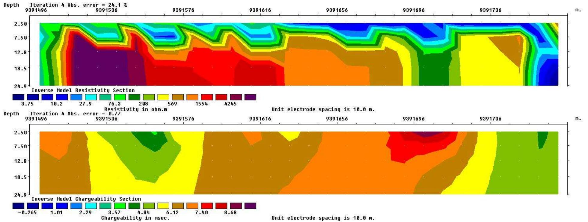
Figure 38: Inverse model resistivity and chargeability sections of line 413087 North
