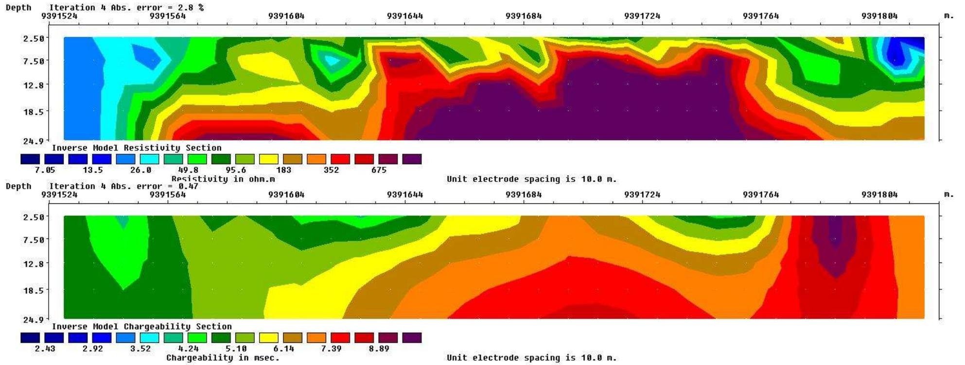
Figure 31: Inverse model resistivity and chargeability sections of line 414187
