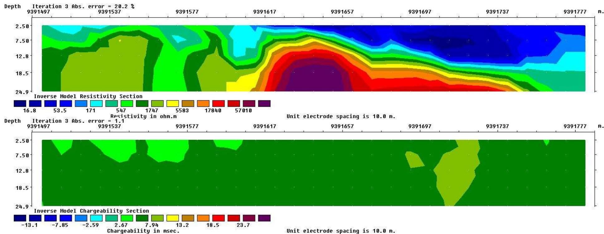
Figure 37: Inverse model resistivity and chargeability sections of line 413087
