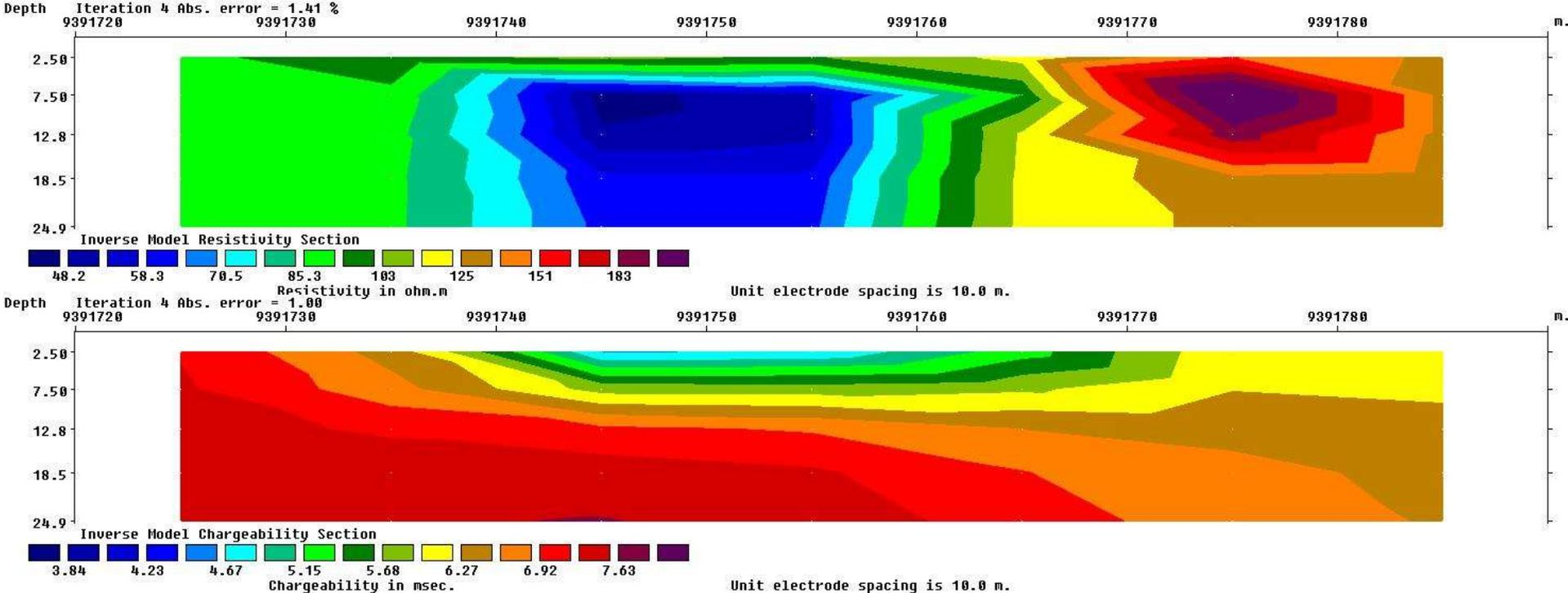
Figure 33: Inverse model resistivity and chargeability sections of line 413237 North
