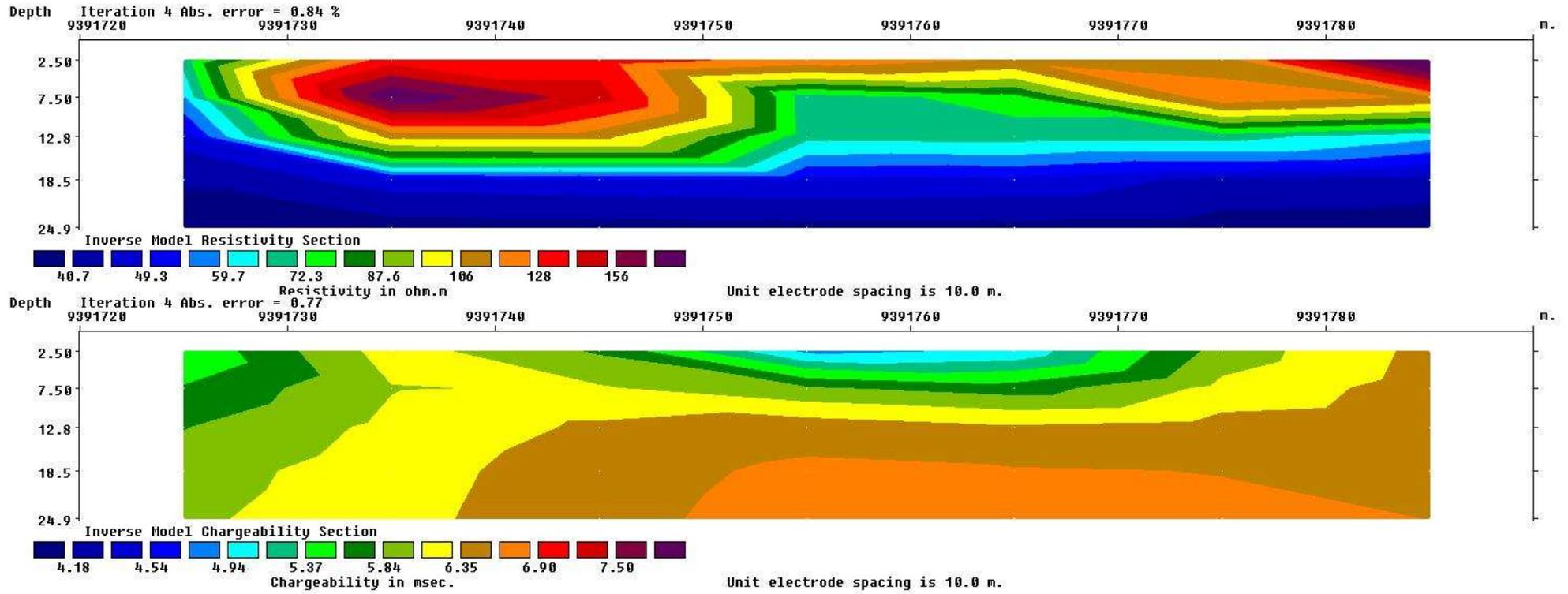
Figure 28: Inverse model resistivity and chargeability sections of line 413337 North
