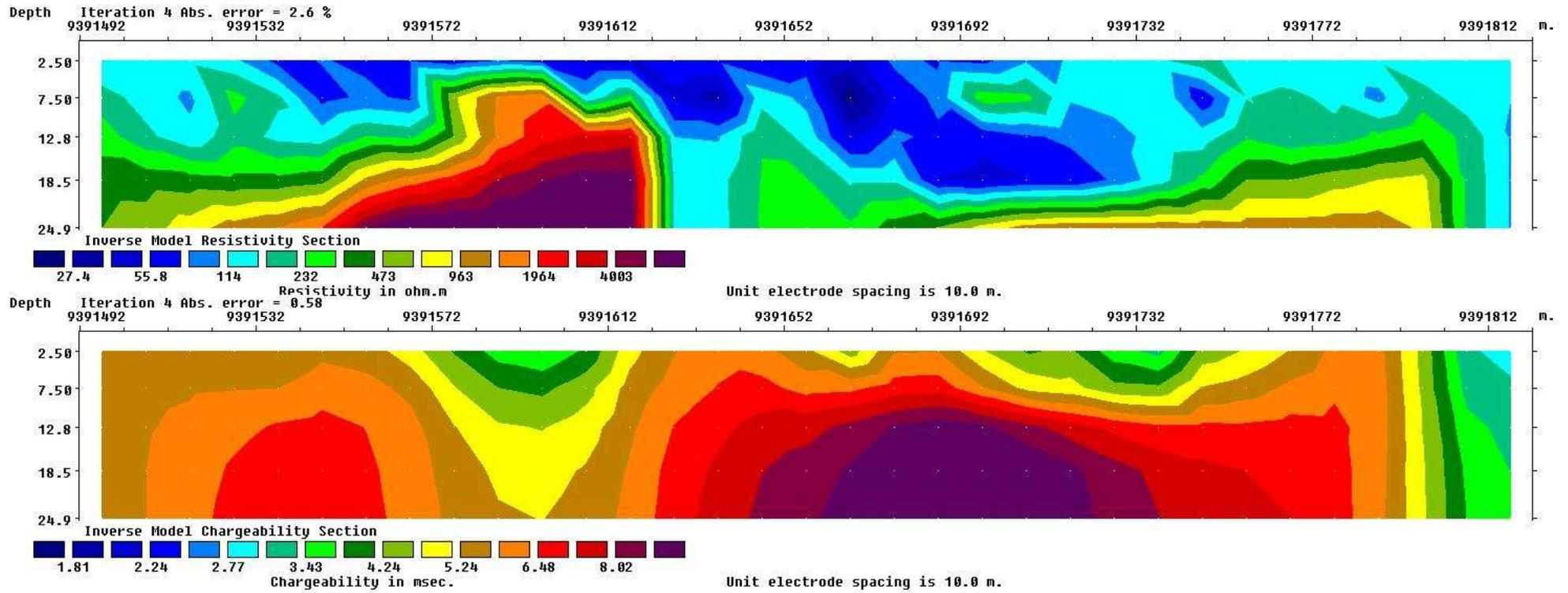
Figure 41: Inverse model resistivity and chargeability sections of line 412937
