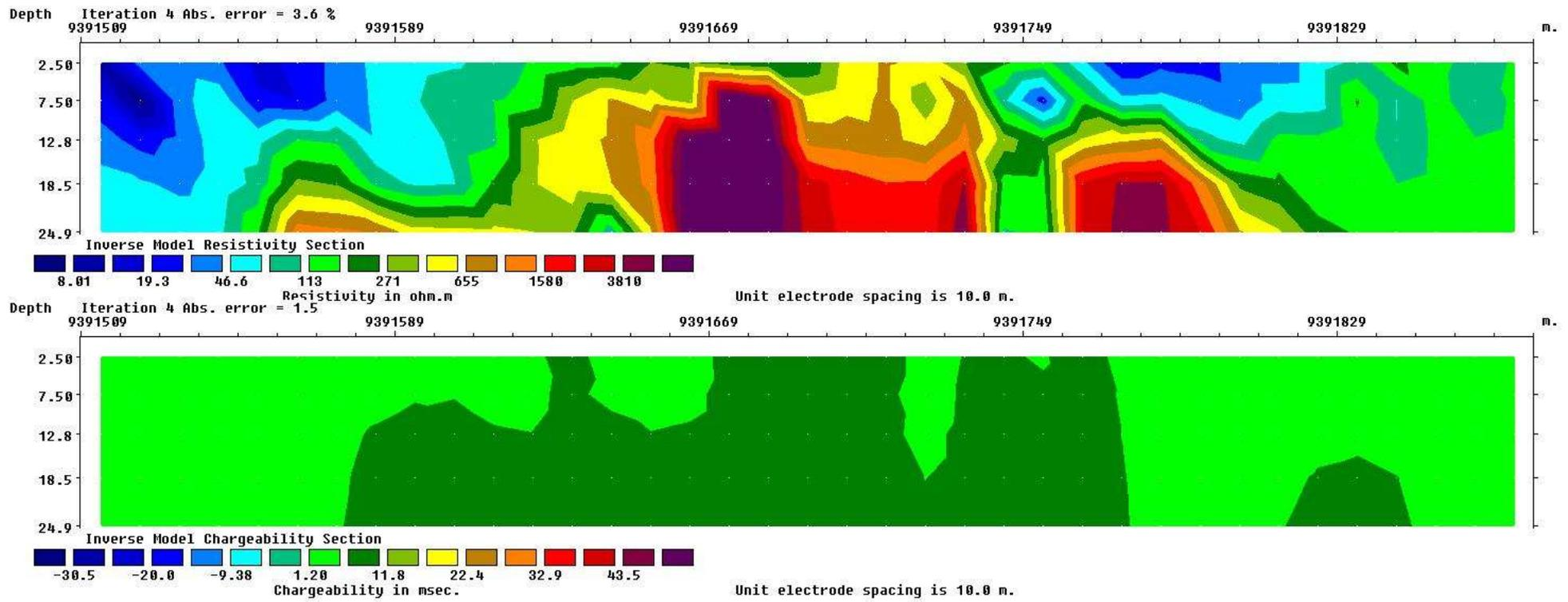
Figure 23: Inverse model resistivity and chargeability sections of line 413587
