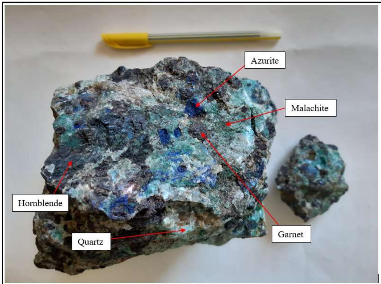
**Figure 7:** Copper ores in the study area; Malachite (light green) and Azurite (deep blue) found in quartz vein
