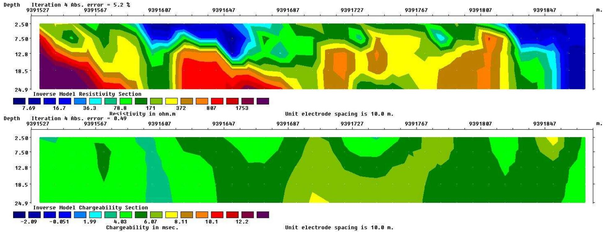
Figure 8: Inverse model resistivity and chargeability sections of line 414337
