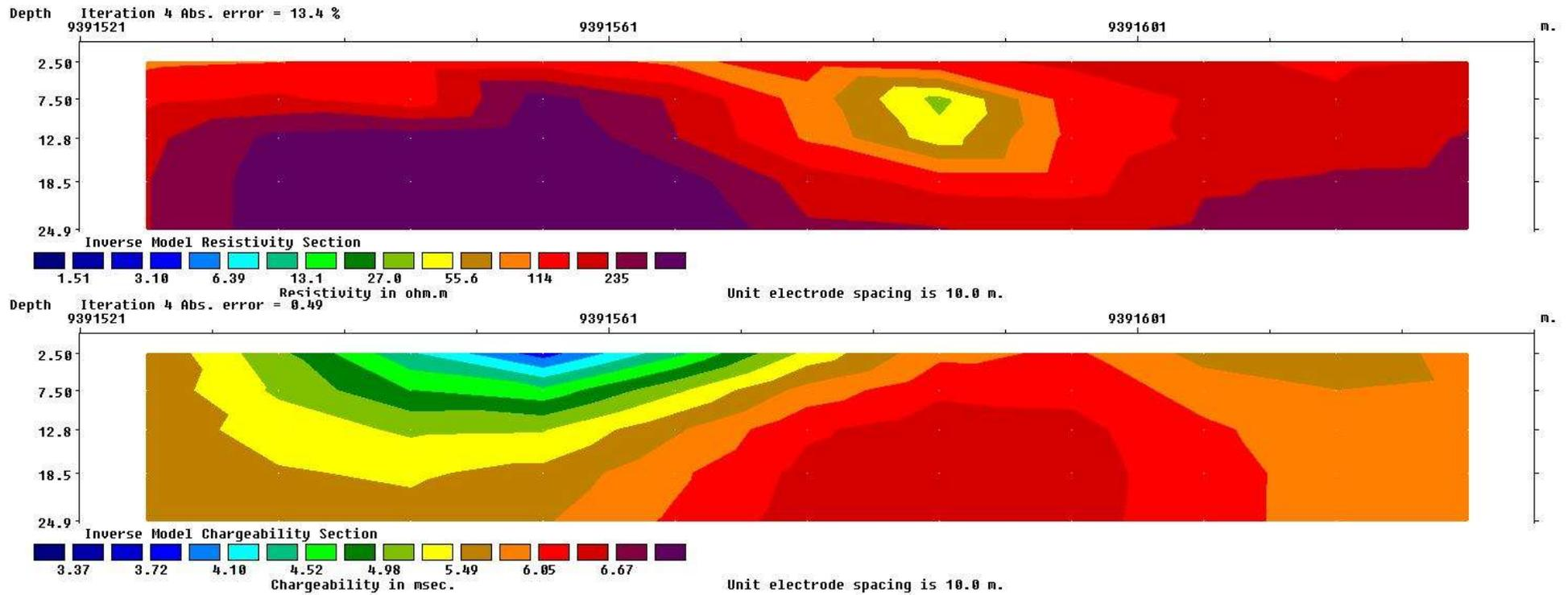
Figure 12: Inverse model resistivity and chargeability sections of line 414087 South
