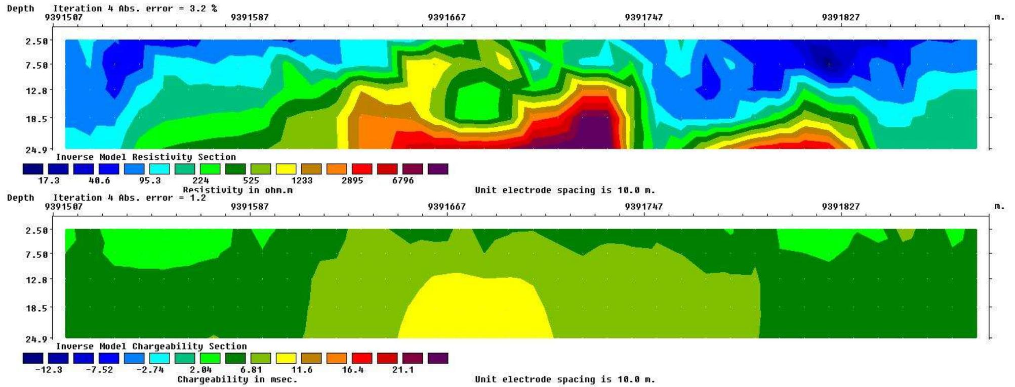
Figure 24: Inverse model resistivity and chargeability sections of line 413587
