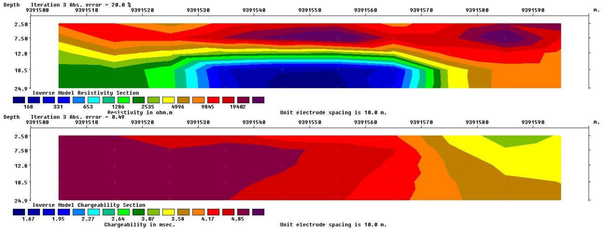
Figure 34: Inverse model resistivity and chargeability sections of line 413237
