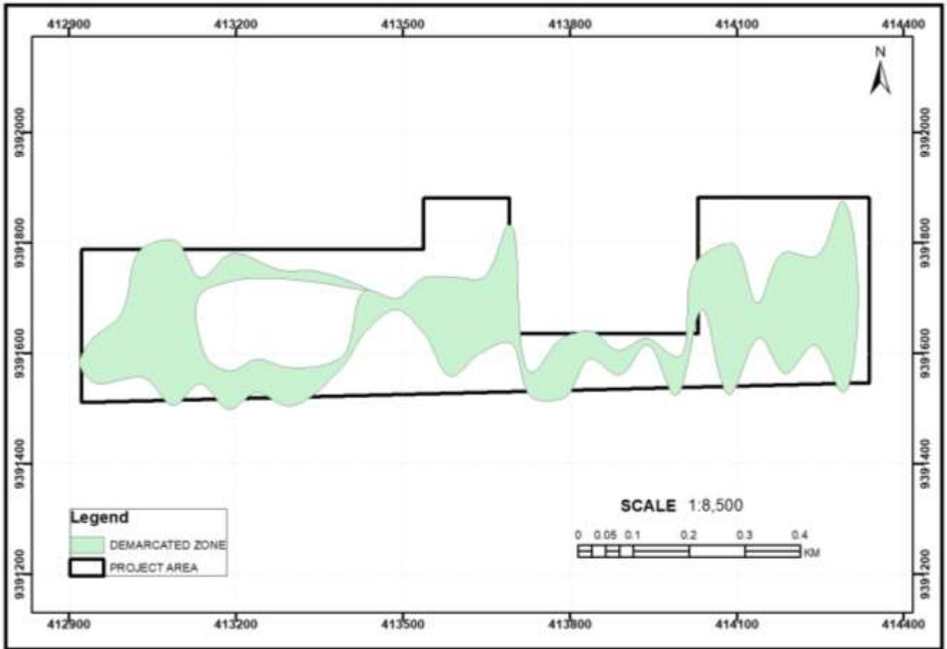
**Figure 42:** Demarcated zone based on IP and resistivity results
