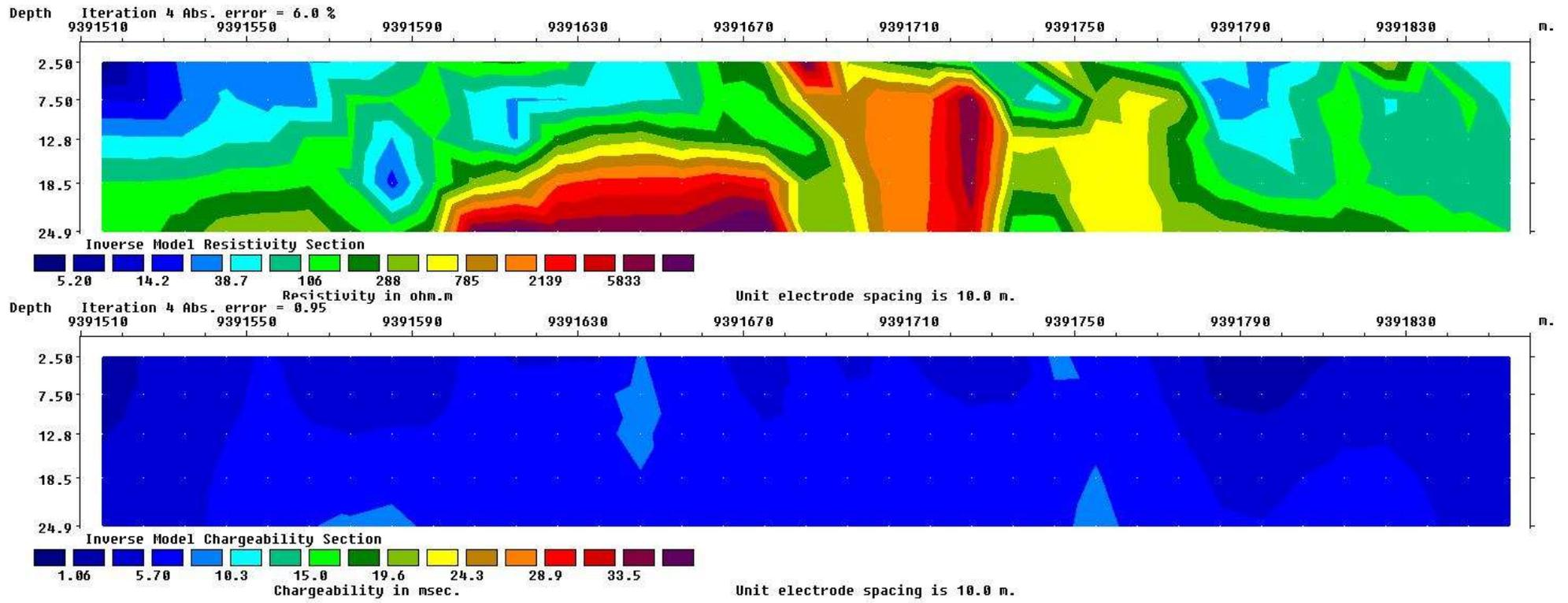
Figure 22: Inverse model resistivity and chargeability sections of line 413637
