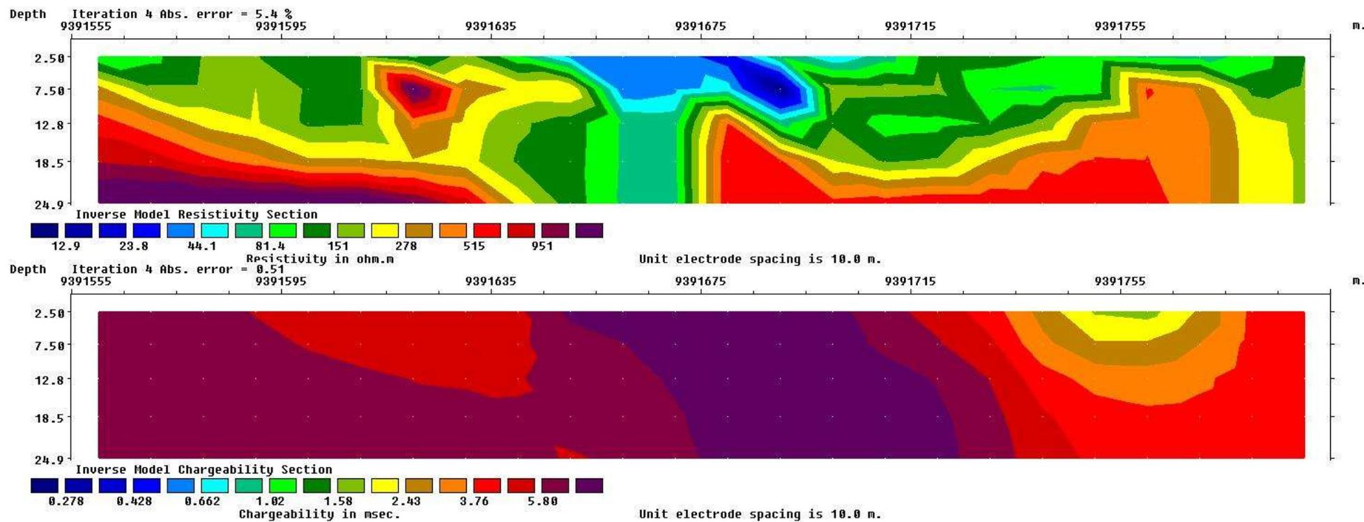
Figure 39: Inverse model resistivity and chargeability sections of line 413037
