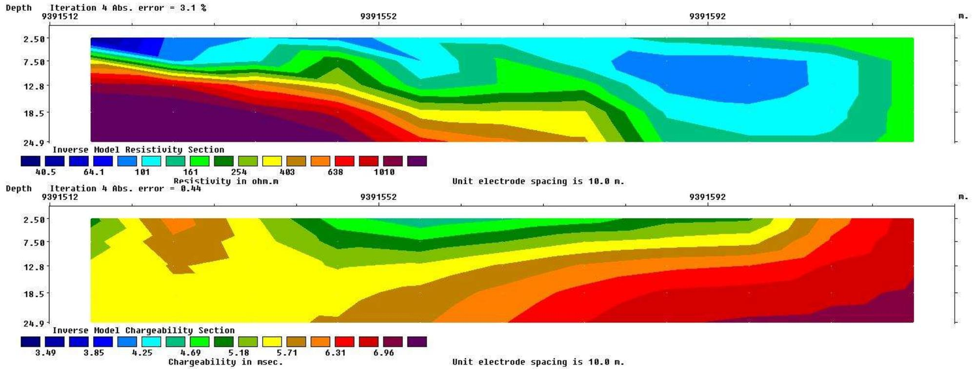
Figure 20: Inverse model resistivity and chargeability sections of line 413737
