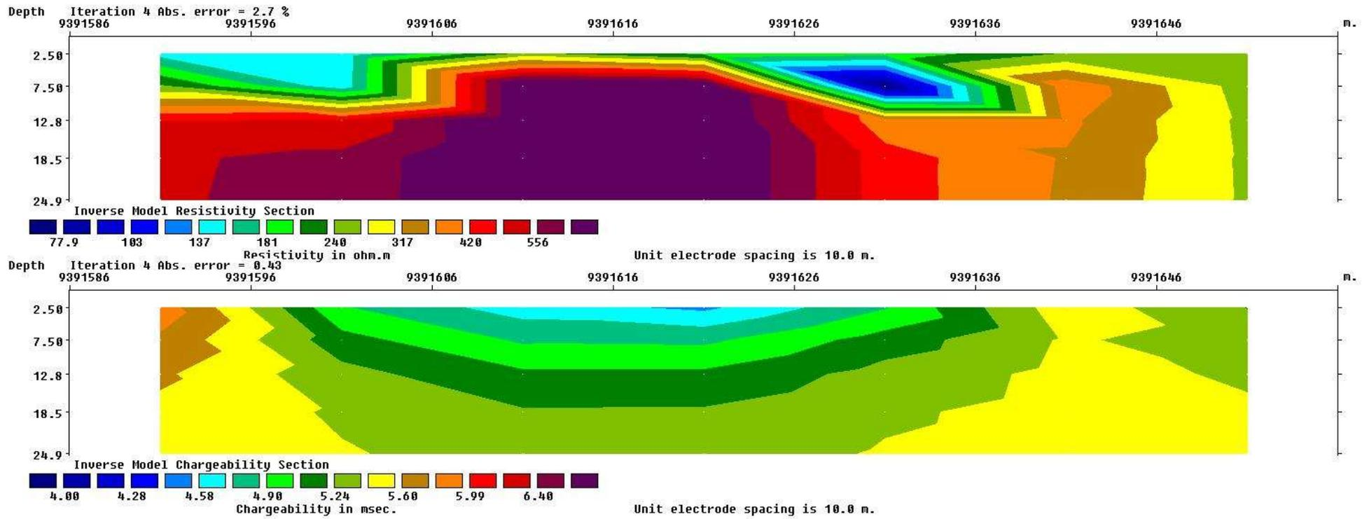
Figure 18: Inverse model resistivity and chargeability sections of line 413837
