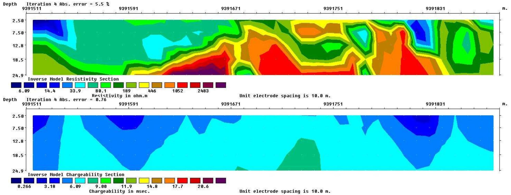
Figure 21: Inverse model resistivity and chargeability sections of line 413687
