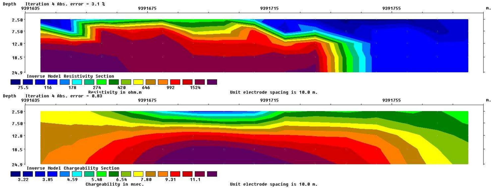
Figure 25: Inverse model resistivity and chargeability sections of line 413487
