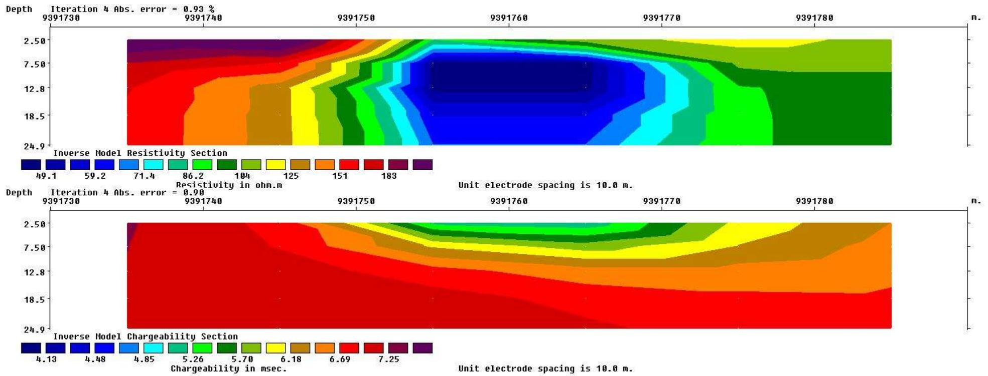
Figure 30: Inverse model resistivity and chargeability sections of line 413287 North
