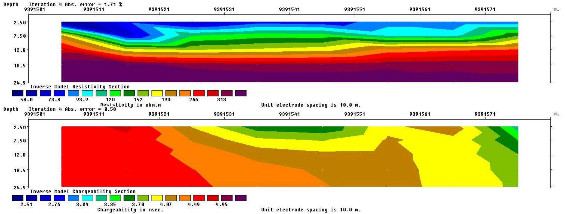
Figure 32: Inverse model resistivity and chargeability sections of line 413287
