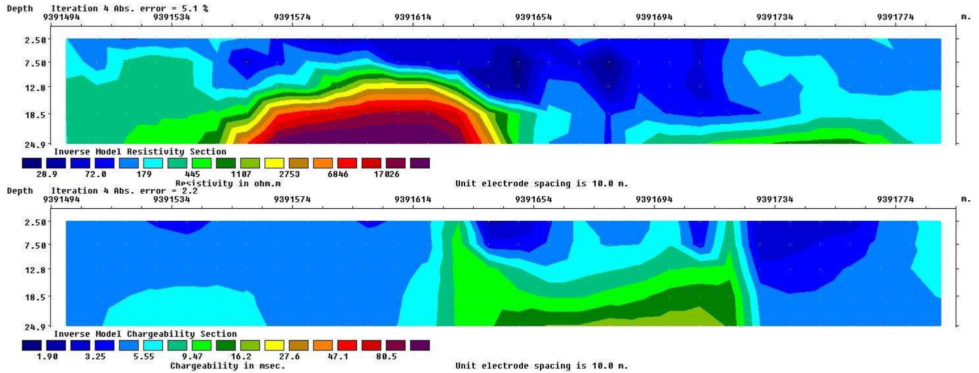
Figure 40: Inverse model resistivity and chargeability sections of line 412987
