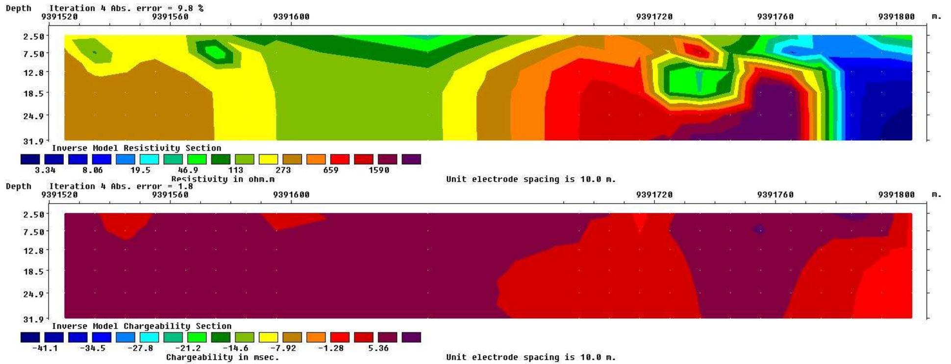
Figure 14: Inverse model resistivity and chargeability sections of line 414037
