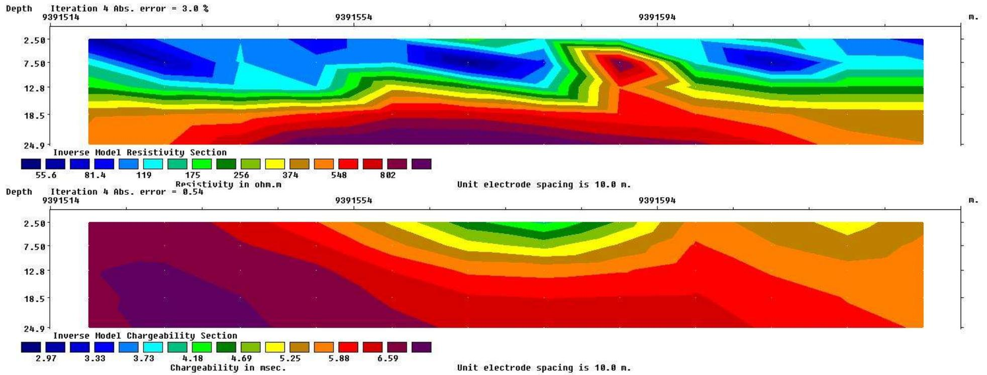
Figure 19: Inverse model resistivity and chargeability sections of line 413787
