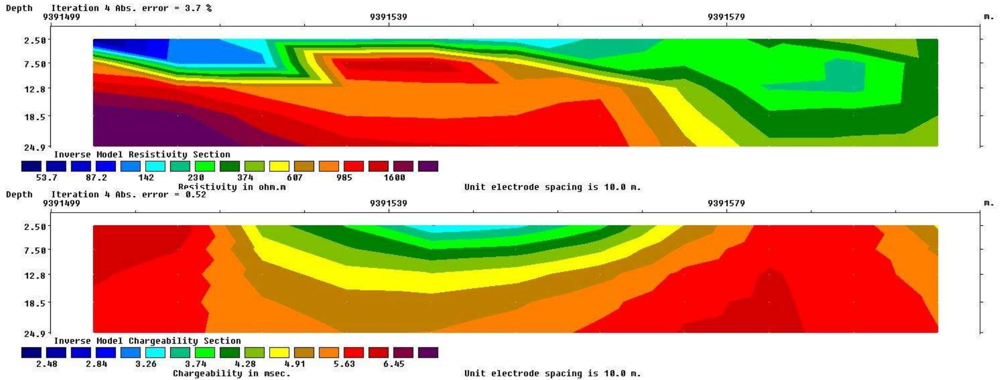
Figure 36: Inverse model resistivity and chargeability sections of line 413187
