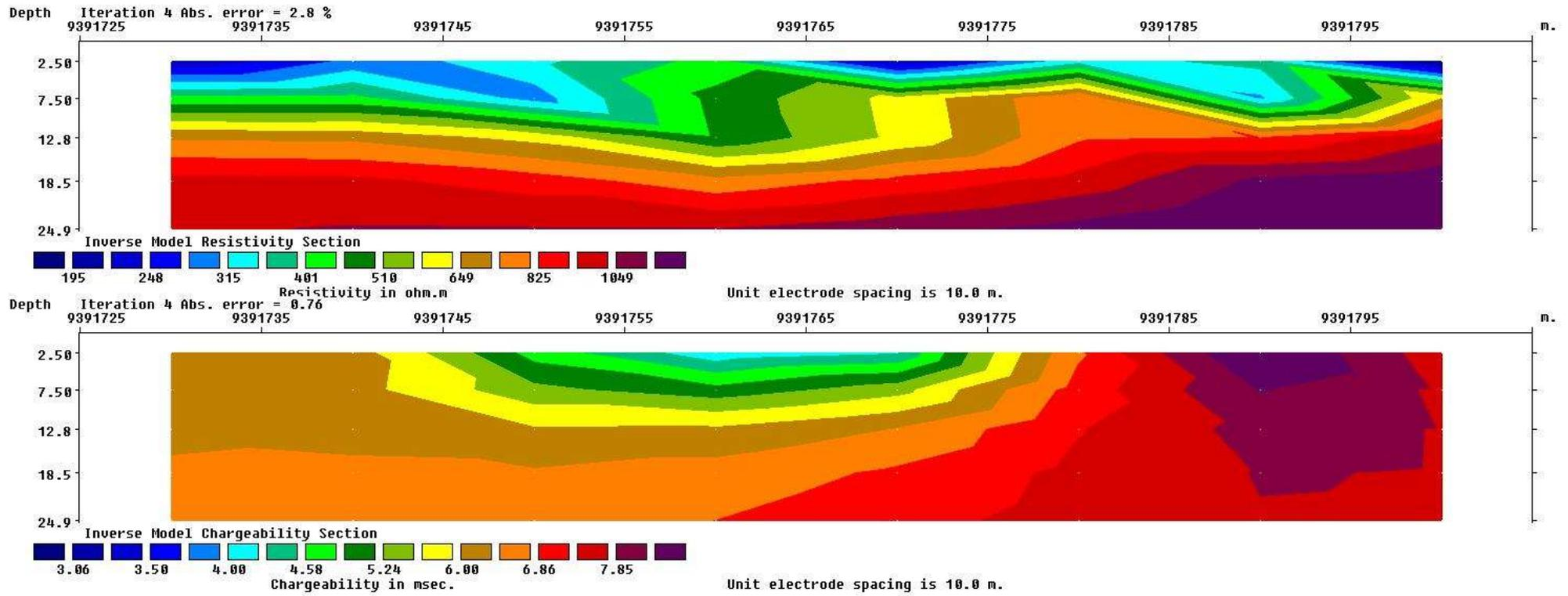
Figure 13: Inverse model resistivity and chargeability sections of line 414087
