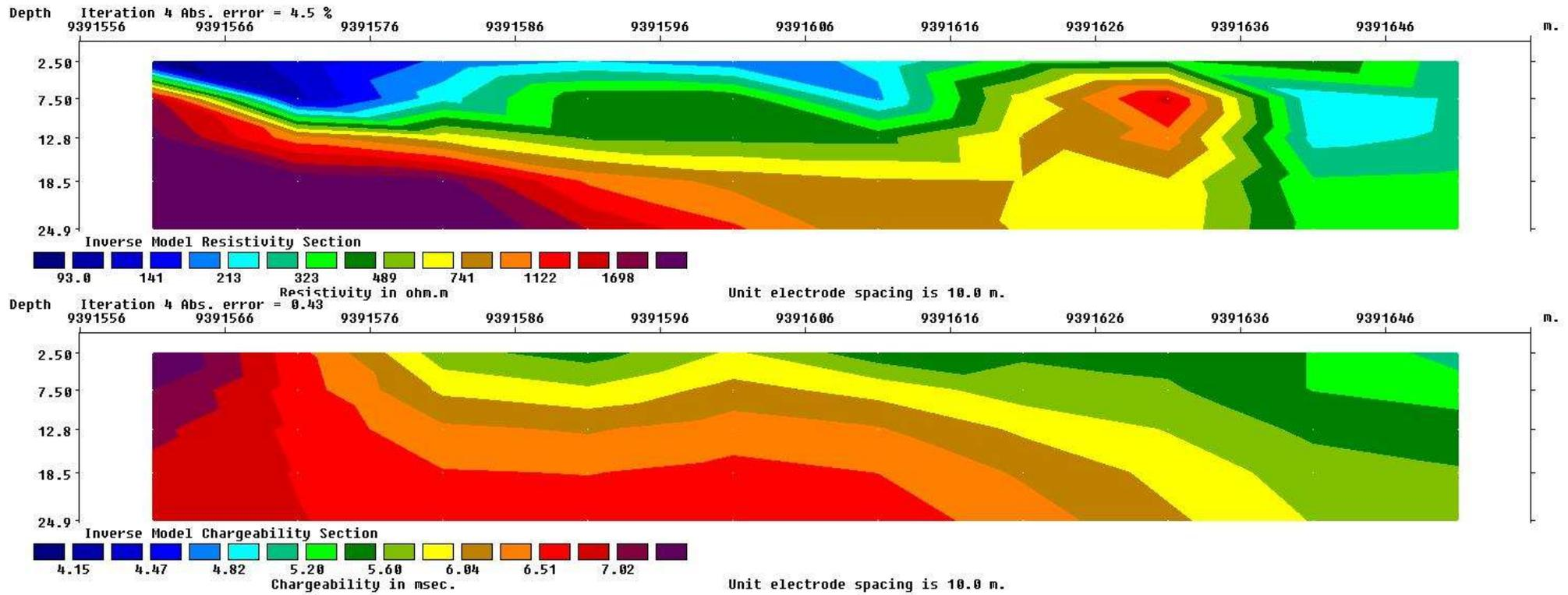
Figure 17: Inverse model resistivity and chargeability sections of line 413887
