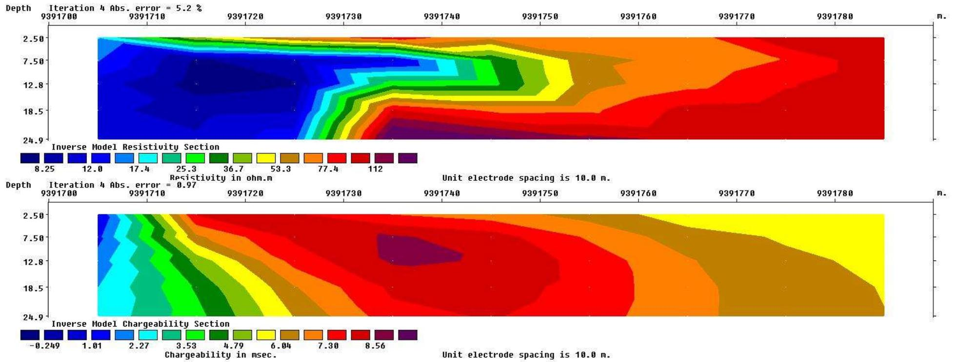
Figure 35: Inverse model resistivity and chargeability sections of line 413187 North
