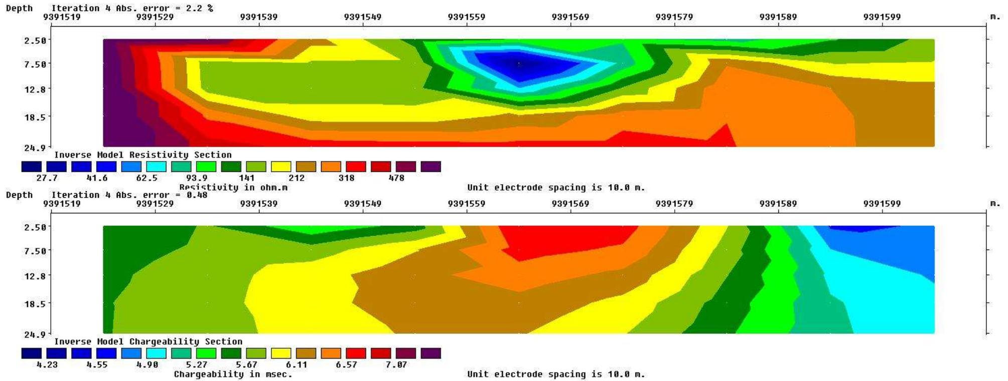
Figure 15: Inverse model resistivity and chargeability sections of line 413987
