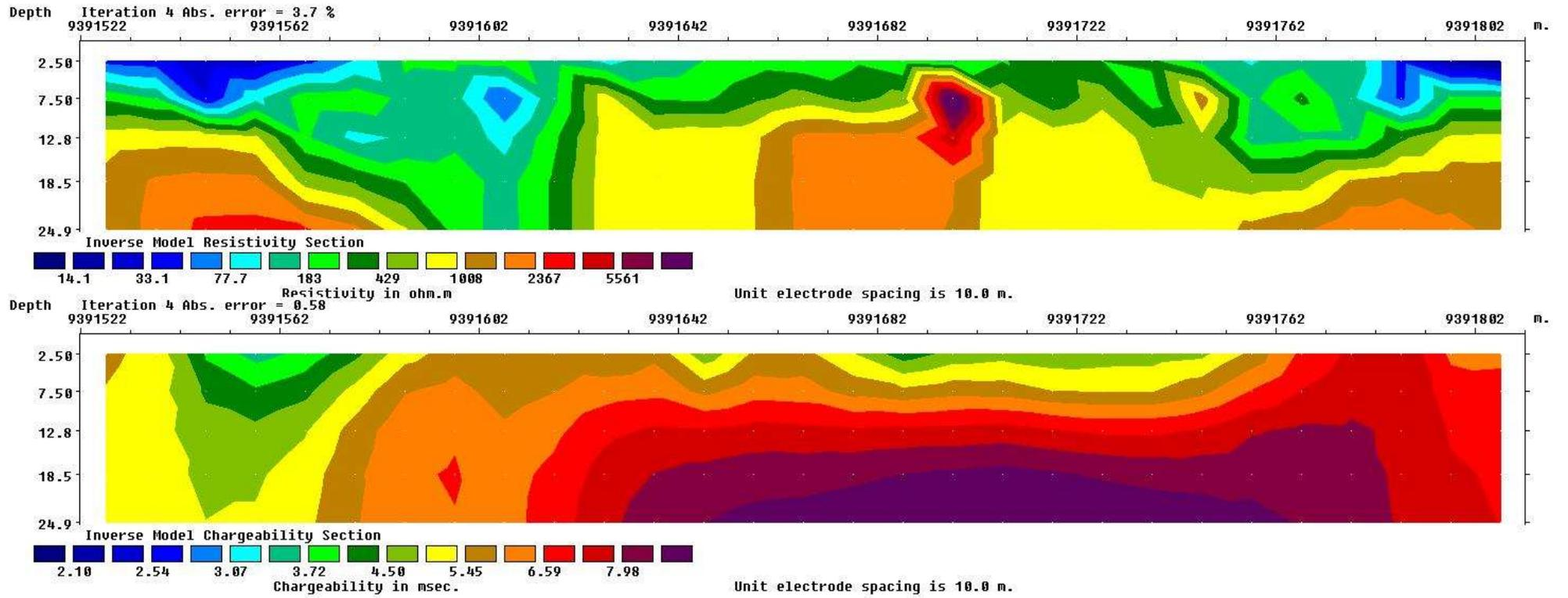
Figure 11: Inverse model resistivity and chargeability sections of line 414137
