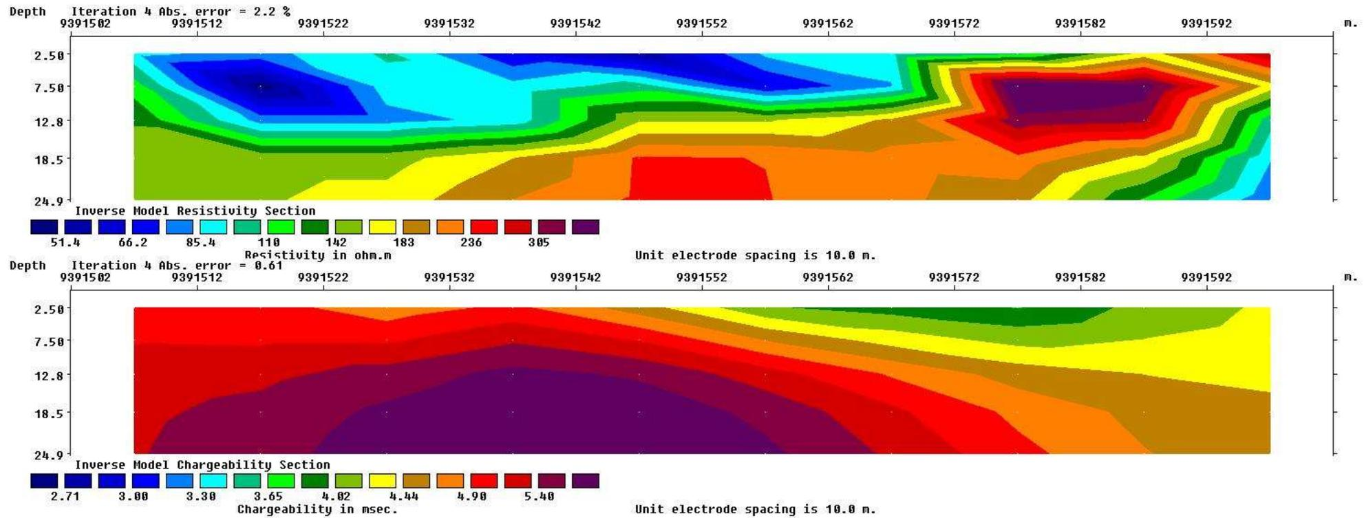
Figure 29: Inverse model resistivity and chargeability sections of line 413337
