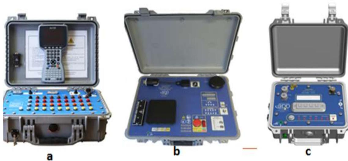
**Figure 3:** (a) IP Receiver GRx 8 – 32 (b) IP Transmitter TX4 5000W (c) EM - IP Tx Controller
