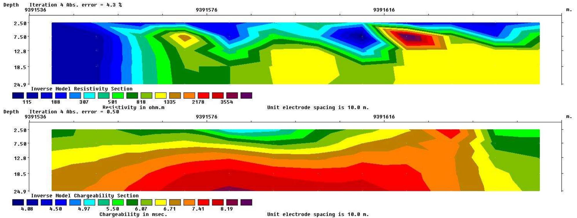
Figure 16: Inverse model resistivity and chargeability sections of line 413937
