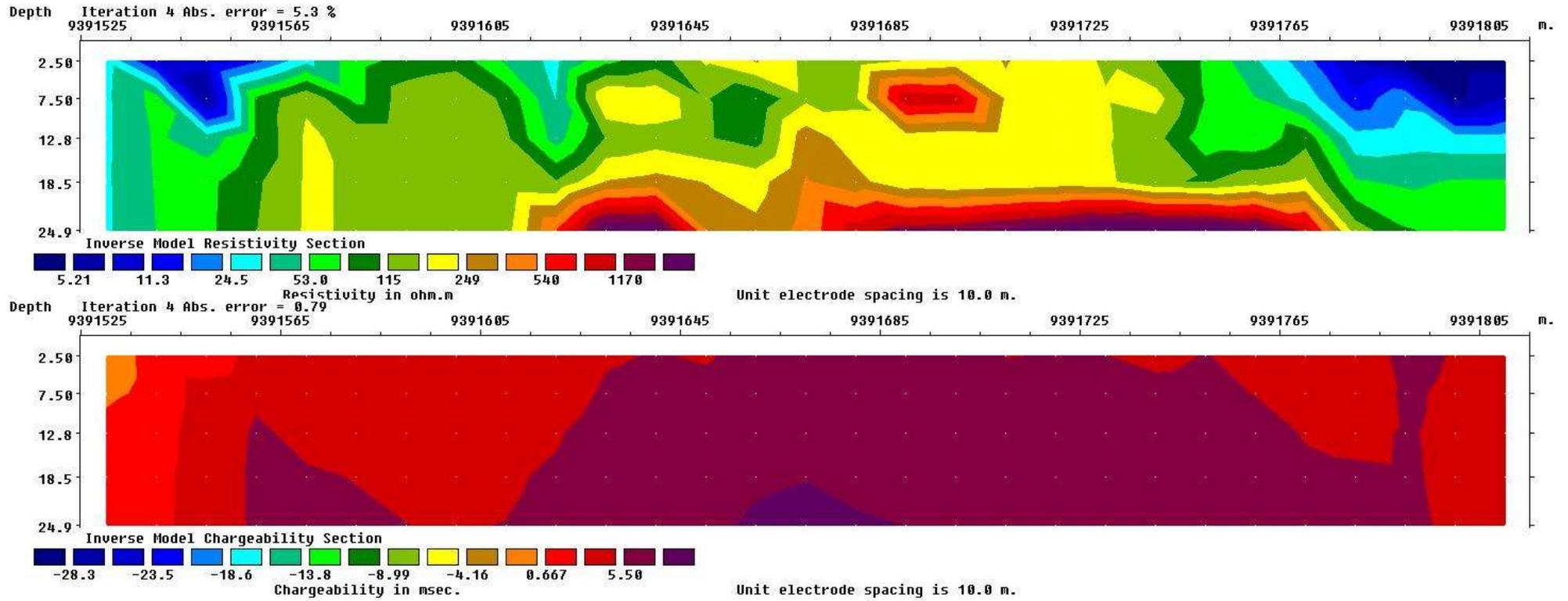
Figure 10: Inverse model resistivity and chargeability sections of line 414237
