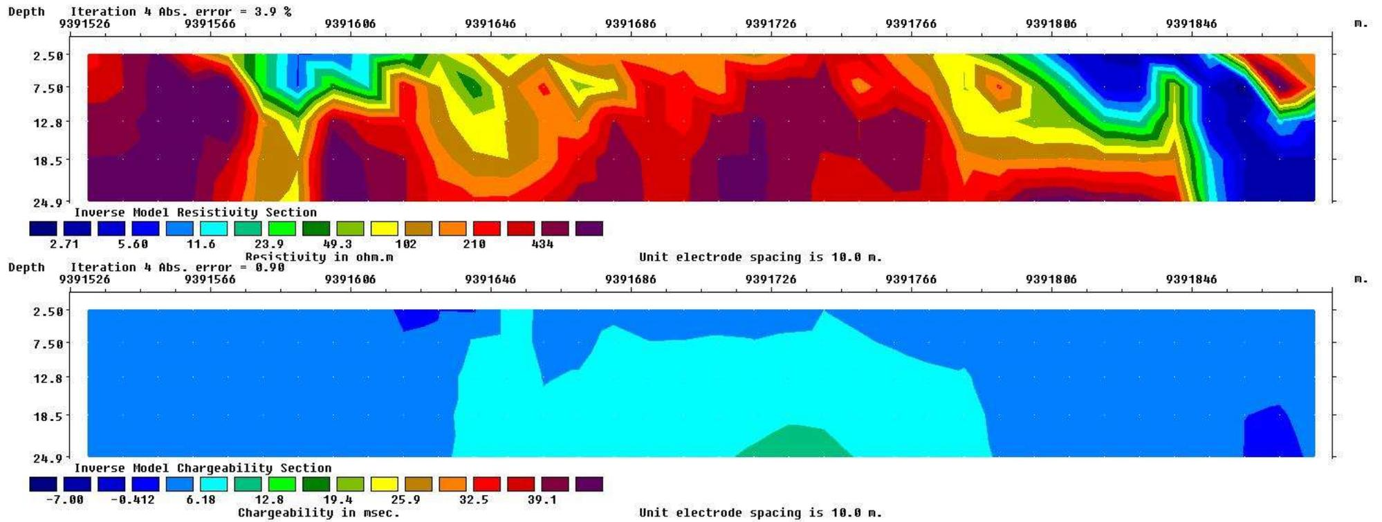
Figure 9: Inverse model resistivity and chargeability sections of line 414287
